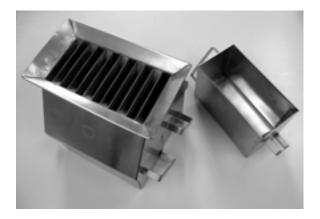
Figure 5.4: Riffle divider for dividing samples in a representative manner
