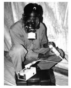
Figure 5.35: Electronic meter being used to estimate phosphine concentration
