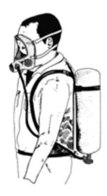
Figure 5.38: Full self-contained breathing apparatus
