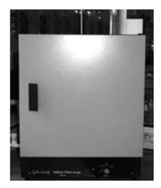
Figure 5.28: A mechanically ventilated oven
