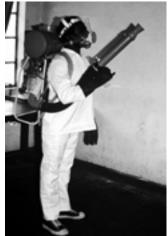
Figure 5.32: Motorised knapsack sprayer in use
