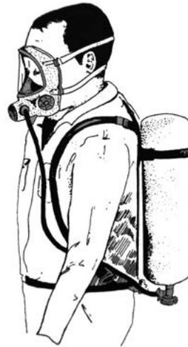
**Figure 5.36: Appareil respiratoire autonome complet**
