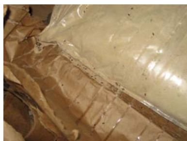
WRONG: Damaged inner layer, infested product
