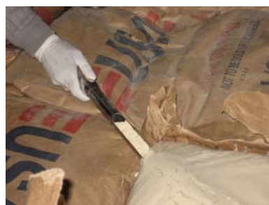
Sampling from the top of the stack
