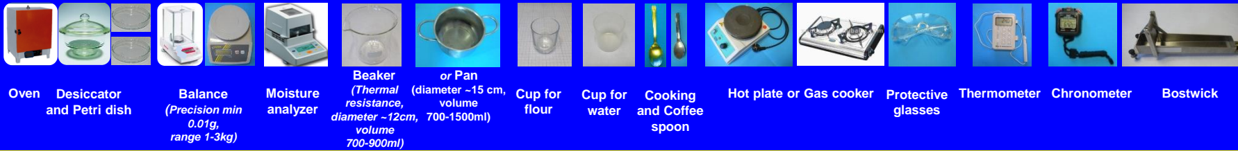
Oven Desiccator and Petri dish Balance (Precision min 0.01g, range 1-3kg) Moisture analyzer Beaker (or Pan) (Thermal resistance, diameter ~12cm, volume 700-1500ml) Cup for flour Cup for water Cooking and Coffee spoon Hot plate or Gas cooker Protective glasses Thermometer Chronometer Bostwick
