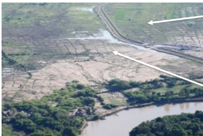
Figure 4.68 - Main damage and clogging of the primary irrigation canal (Artibonite, 2008 – Haiti, source WFP, V. Carucci). Irrigation fields destroyed and in need of major rehabilitation.
