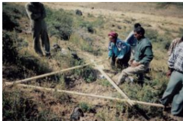
Using A-frame for layout and design of trenches
