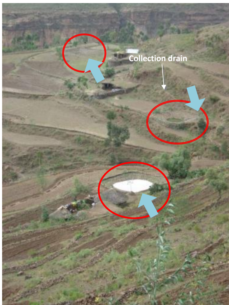
Figure 4.4 - Micro-ponds collecting runoff water originating from stabilized slopes and micro-catchments.
