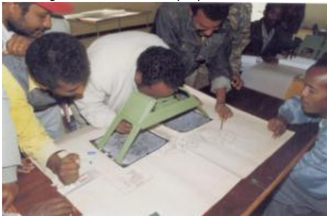
Using aerial photos & stereoscopes for mapping
