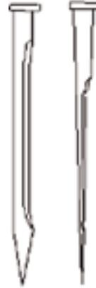
**Figure 5.1: Bag sampling spears (left to right) - cylindrical spear, tapered spear**
