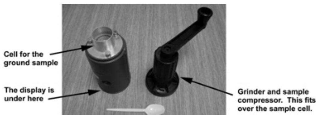
**Figure 5.26: A resistance type moisture meter**
