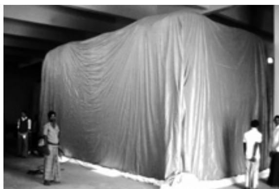
**Figure 5.30: A bag stack placed under gas tight sheets ready for fumigation to proceed**
