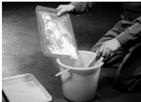
**Figure 5.42: Mixing phosphine residues with water to de-activate them**
