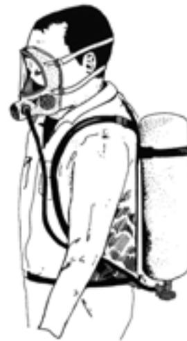
**Figure 5.38: Full self-contained breathing apparatus**
