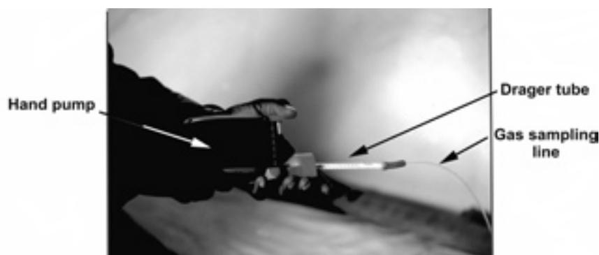
**Figure 5.34: Hand pump with Dräger tube for estimation of phosphine concentration. A gas sampling line is fixed to the Dräger tube so that gas can be drawn from beneath the fumigation sheet.**
