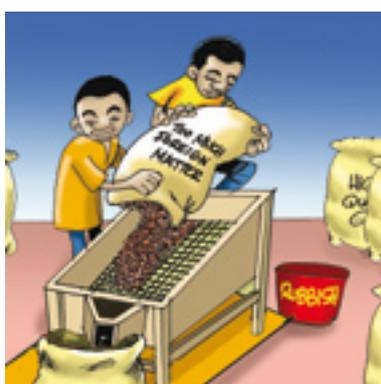
*Empty the grain onto an inclined sieve*
