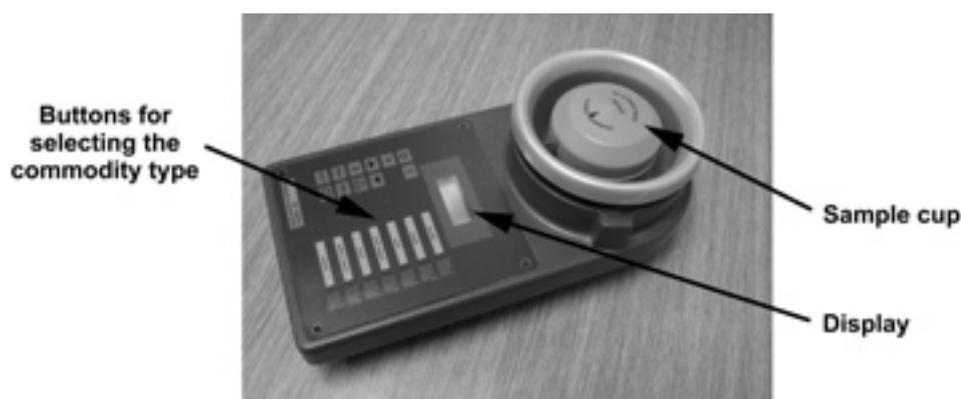
**Figure 5.27: A capacitance type moisture meter**
