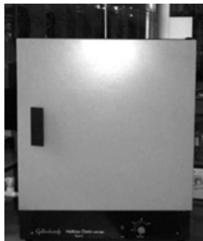
**Figure 5.28: A mechanically ventilated oven**
