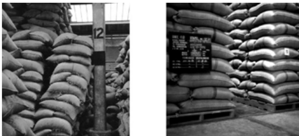
**Figure 5.39: An example (left) of an insecurely built bag stack with bags not properly 'stacked/ keyed' and closer than 1.5m to a pillar, compared with a well-constructed bag stack (right) with a good 1.5m alley separating it from an adjacent stacks.**
