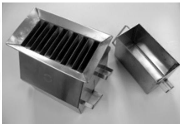
**Figure 5.4: Riffle divider for dividing samples in a representative manner**
