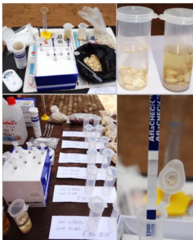
Illustration E: Aflatoxin testing in the field: Using processional equipment to test reactions between antibodies and aflatoxin in stored crop samples. The tests indicated where aflatoxin levels had exceeded the defect action level of 20 ppb.
